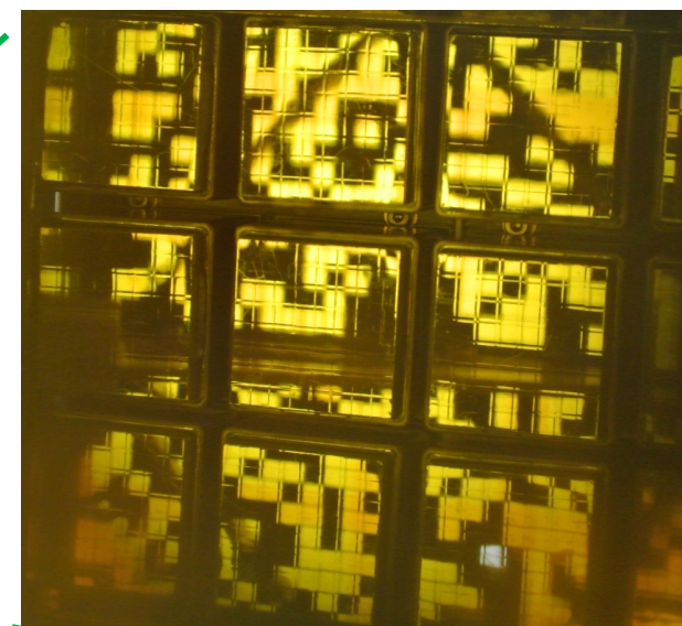
Coded mask pattern on UBAT detector plane
